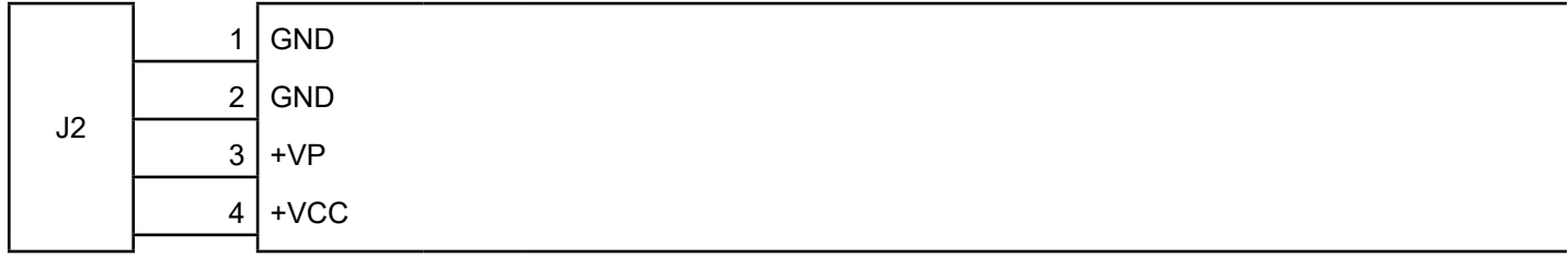
POWER SUPPLY JST male connector (S4B-PH-K-S)
